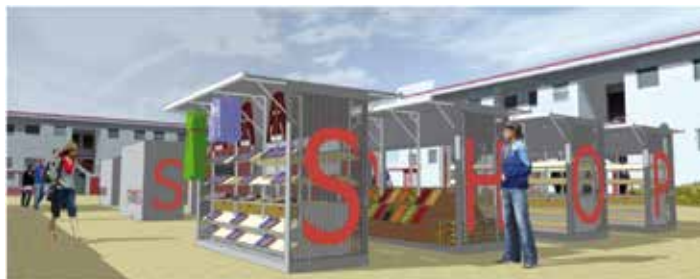
Fixed market (semi-folded units to gain space after closing time) for street vendors with large heavy products in order to legalise their situation. Dr Magdy Mousa
